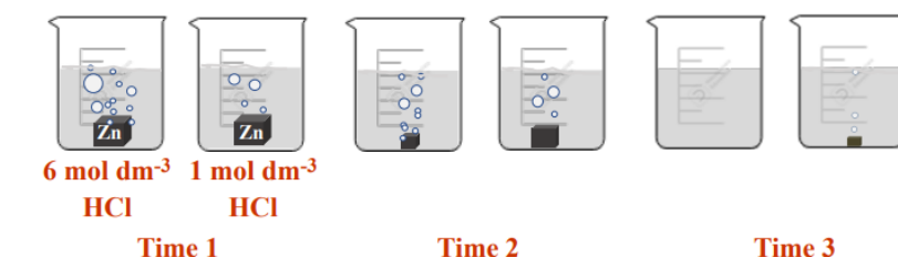
Figure 3.5 The Progress of Reactions of Zn with Different Concentrations of HCl during Three Periods of Time
