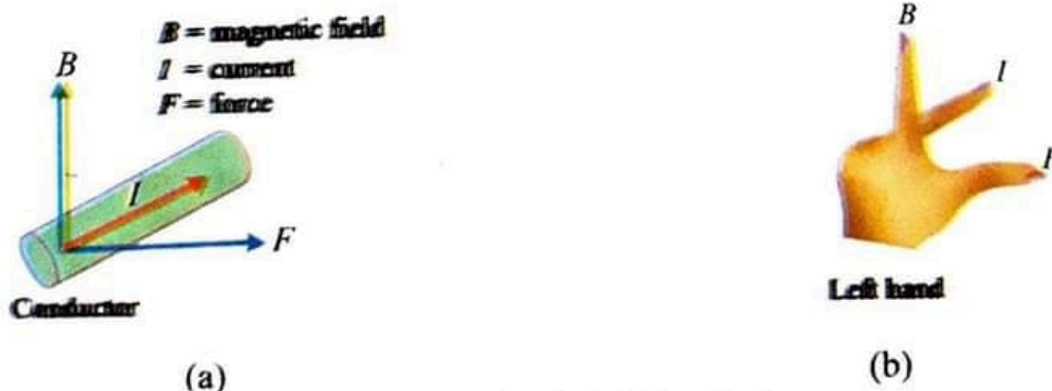
Figure 10.16 Fleming's left-hand rule
