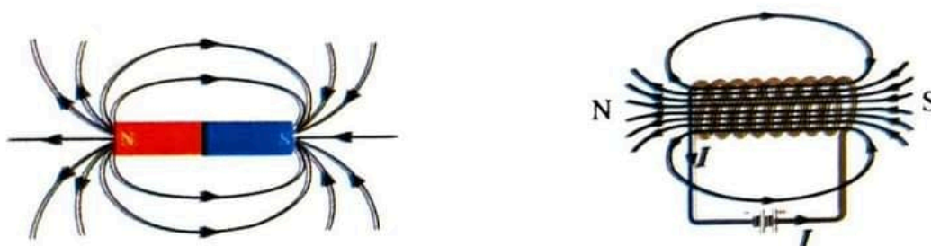
Figure 10.15 Magnetic field of a solenoid
