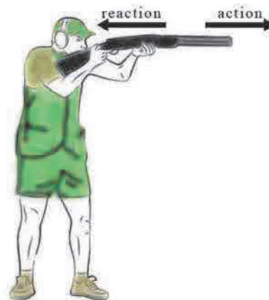
Figure 3.3 Action and reaction force for firing a gun
